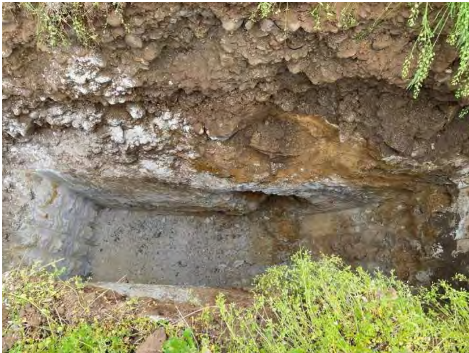
Photograph 6 Test pit with non-indigenous fill material
